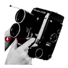
Insert the lens into the lens mount so that the lens shutter cocking lever (4) connects with the cocking lever on the camera body. This operation is more easily performed by cocking the lens shutter with the fingers and inserting the lens from the cocking lever side on the body.
